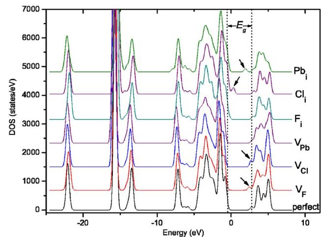
FIG. 7. (Color online) Densities of states for neutral perfect and defective PbFCl supercells. The arrows denote the extra levels in the band gap.
