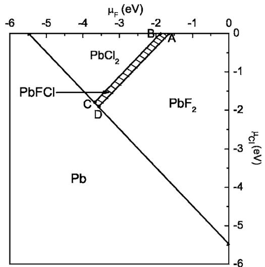
FIG. 2. The calculated stability quadrangle for Pb-F-Cl systems in the μ<sub>F</sub>, μ<sub>Cl</sub> plane. The dashed zone represents the region of stability of PbFCl. The lines AD and BC are determined by Eqs. (5) and (6), respectively.
