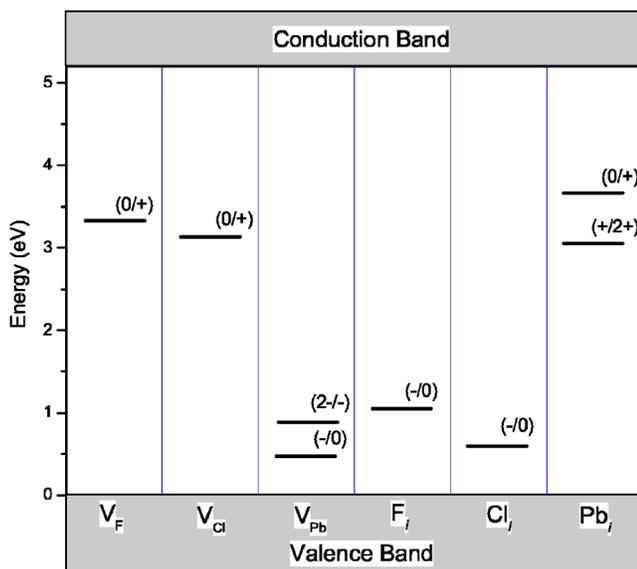
FIG. 6. (Color online) Calculated defect transition energy levels  $\epsilon_{\alpha}(q/q')$  according to Eq. (3).
