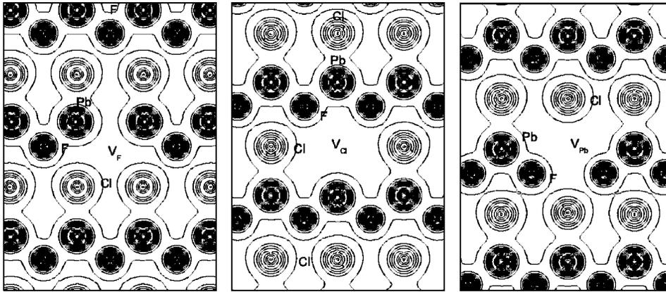
FIG. 5. Contour plot of calculated charge density of vacancy-containing PbFCl. The contour lines are from 0.07 to 11.3  $e/\text{\AA}^3$  with an interval of 0.4  $e/\text{\AA}^3$ .
