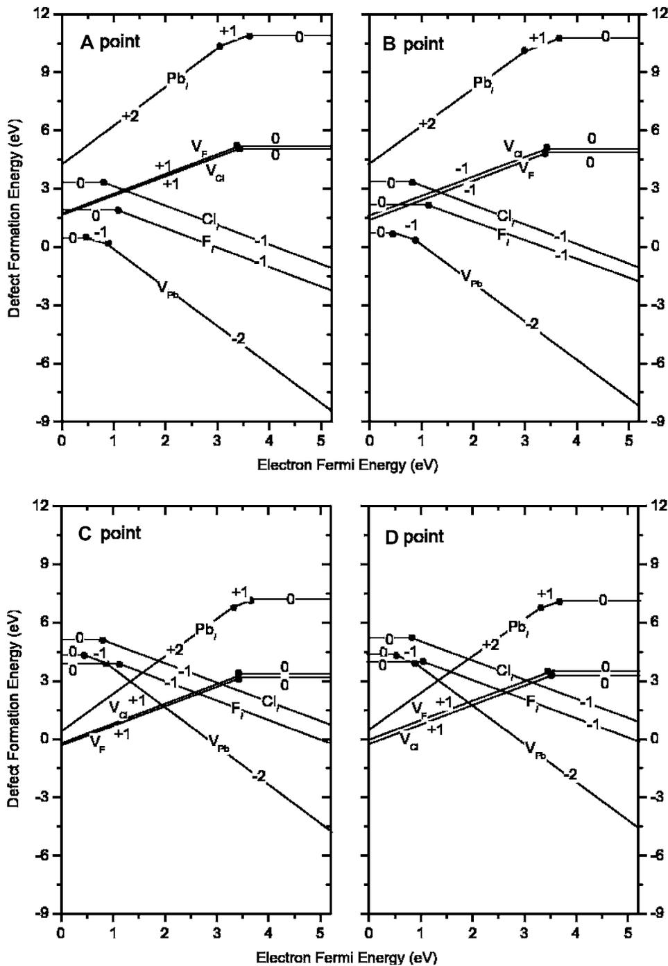
FIG. 4. Formation energies as a function of the electron Fermi energy  $E_F$  at atomic chemical potentials A, B, C, and D shown in Fig. 2. The signed numbers stand for the charge states of the defects. Solid dots denote the values of  $E_F$  where transition between charge states happens.
