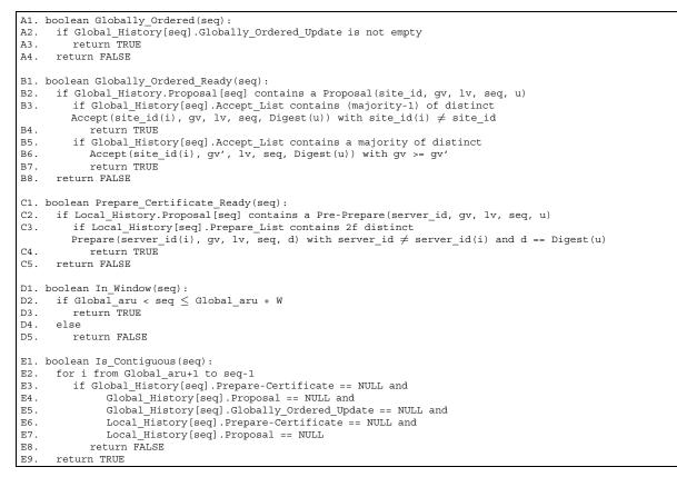
Fig. A-5: Predicate functions used by the global and local protocols to determine if and how a message should be applied to a server's data structures.
