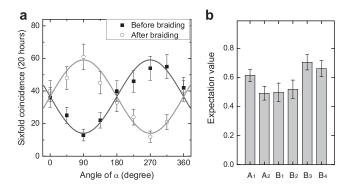
FIG. 4. (a). Measured fringes for the state  $|\psi_s\rangle_6$  and  $|\psi_f\rangle_6$ . Two sinusoid curves are fitted to the data with visibilities of 0.61. The measurements in basis  $(|+\rangle + e^{i\alpha}|-\rangle)$  are done using a combination of HWPs, QWP, and PBS. (b). The expectation values of the operators  $A_1, \dots, B_4$  of the state  $|\psi_f\rangle_6$  after the  $\sqrt{Z_3}$  transformation.
